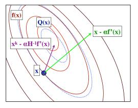
• If  $\nabla^2 f(x)$  is Lipschitz-continuous and  $\nabla^2 f(x) \succeq \mu$ , then close to  $x^*$  Newton's method has local superlinear convergence:
